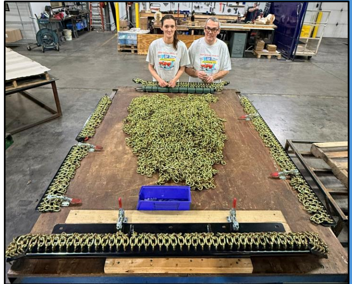
Above: Chrissy Hartman and Ronnie Hatton display a repurposed table with new toggle clamps setup to hold frames at specific angles for chain and cable insertion.
